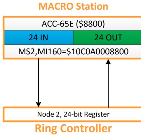
Having downloaded the above settings into the MACRO16 station, the inputs can be read and outputs can be transferred from the ring controller side (I/O node 2) in the following bit fields:
