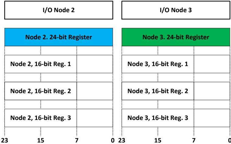
The inputs are mapped into the 24-bit register of node 2
