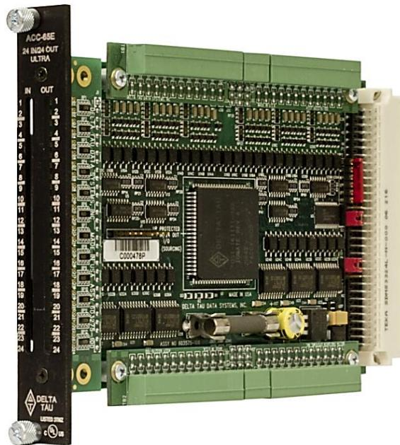
Digital I/O – Sinking Inputs, Sourcing Outputs
