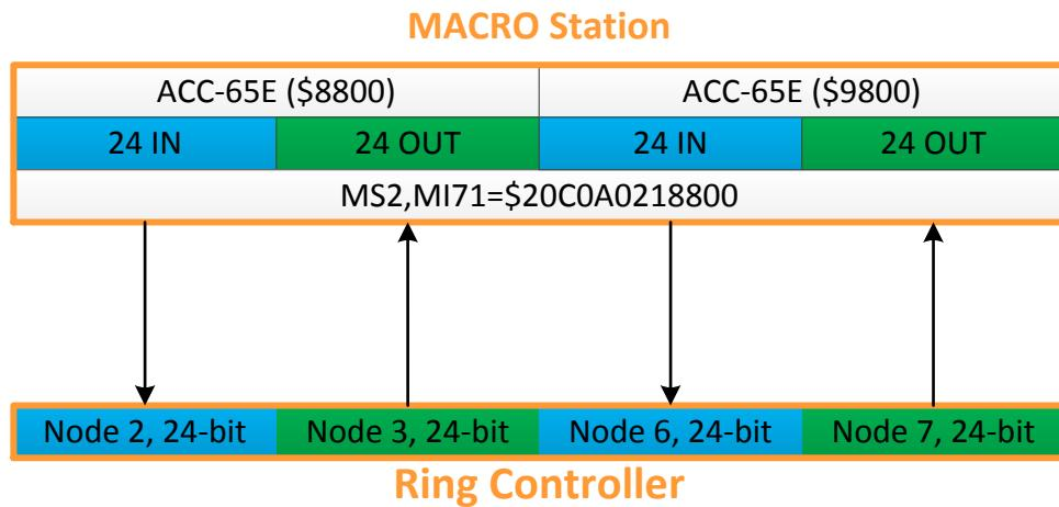
Having downloaded the above settings into the MACRO16 station, the inputs and outputs are now available to access from the ring controller side (e.g. I/O nodes 2, 3, 6, and 7) in the following bit fields:
