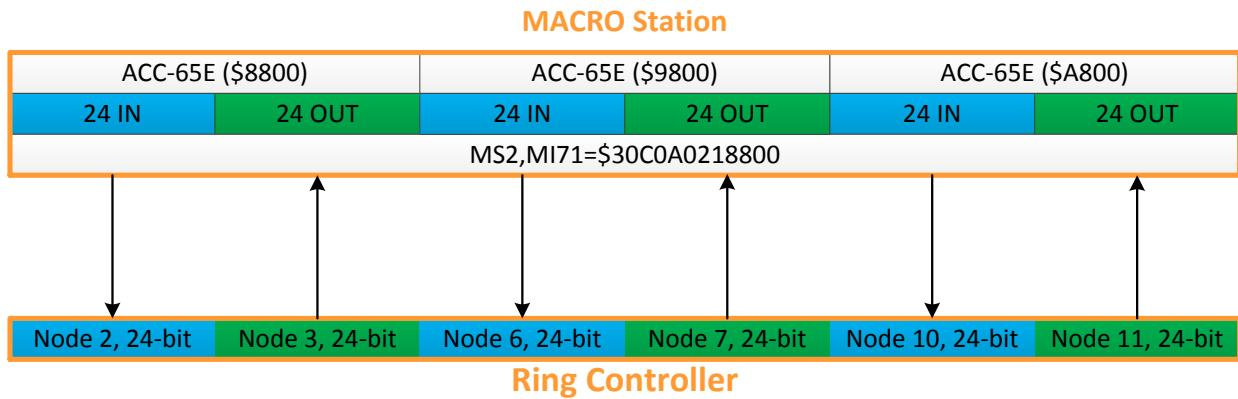
Having downloaded the above settings into the MACRO16 station, the inputs and outputs are now available to access on the ring controller side (I/O nodes 2, 3, 6, 7, 10, and 11) in the following bit fields:
