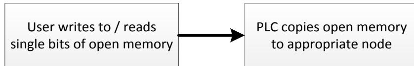
Bitwise mapping to user memory structure elements in Power PMAC is not allowed. Explicit syntax with offset address must be used. The offset address is found by multiplying the element structure index by 4. To the right is an example of the first 4 unsigned open memory structure elements and their corresponding address offsets:
