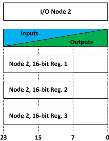
The inputs are mapped into the 24-bit register of node 2
