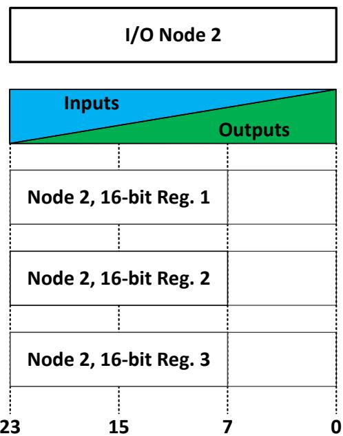
The inputs are mapped into the 24 bits of node 2:
