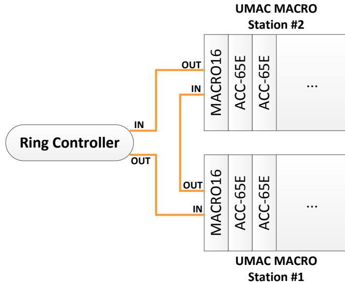
Generally, the user's goal is to transfer the ACC-65E I/O data (48 bits per card) from/to the ring controller by reading the 24-bits of inputs and writing to the 24-bits of outputs.
