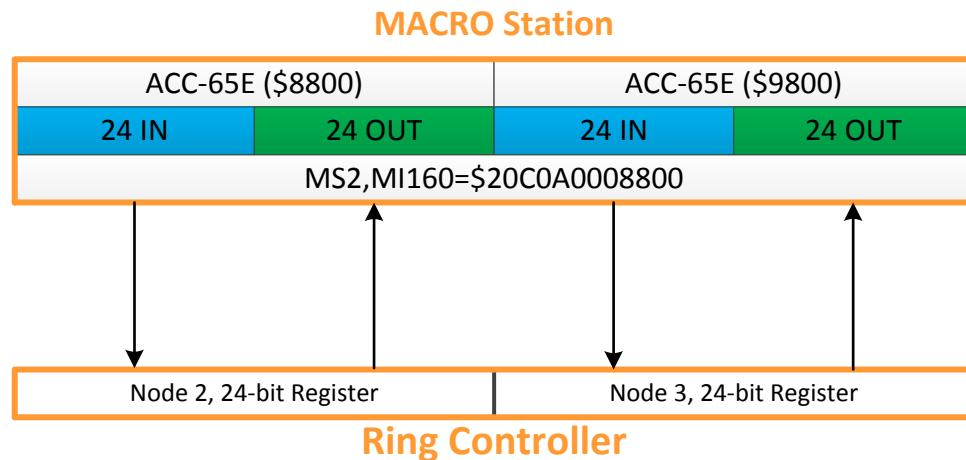
Having downloaded the above settings into the MACRO16 station, the inputs can be read and outputs can be transferred from the ring controller side (I/O nodes 2 and 3) in the following bit fields:
