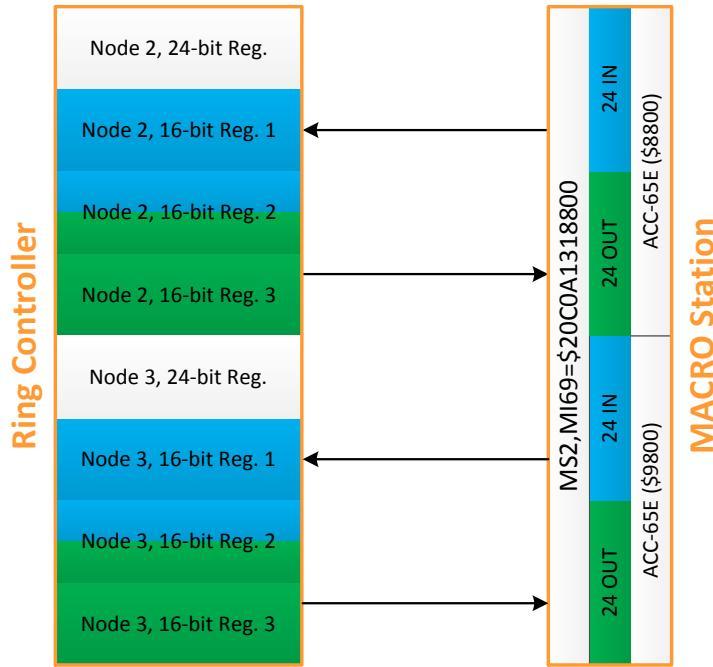
Having downloaded the above settings into the MACRO16 station, the inputs and outputs are now available to access on the ring controller side (I/O nodes 2 and 3) in the following bit fields:
