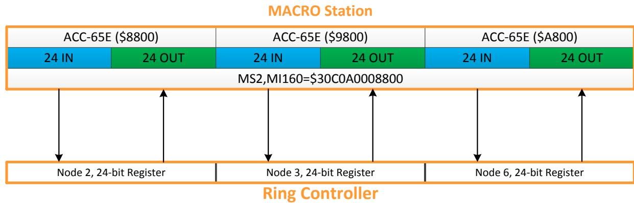
Having downloaded the above settings into the MACRO16 station, the inputs can be read and outputs can be transferred from the ring controller side (I/O nodes 2, 3, and 6) in the following bit fields:
