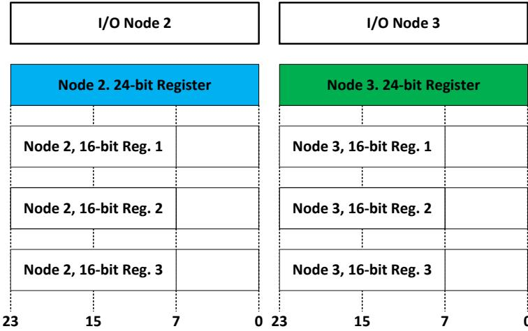
The inputs are mapped into the 24 bits of node 2:
