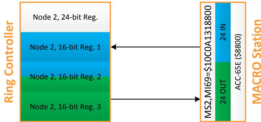
Having downloaded the above settings into the MACRO16 station, the inputs and outputs are now available to access on the ring controller side (I/O node 2) in the following bit fields:
