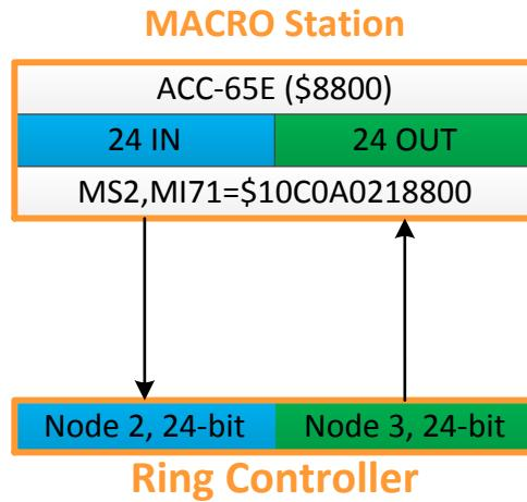
Having downloaded the above settings into the MACRO16 station, the inputs and outputs are now available to access from the ring controller side (e.g. I/O nodes 2, 3) in the following bit fields:
