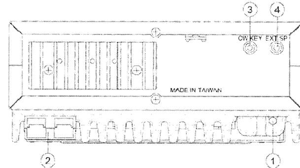
1. **ANTENNA:** This jack accepts a 50 ohms coaxial cable with a PL-259 style plug.
