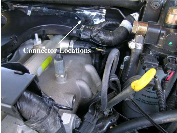
connector into the stock engine MAP sensor and the stock engine wiring harness connector into the supplied MAP sensor connector.
