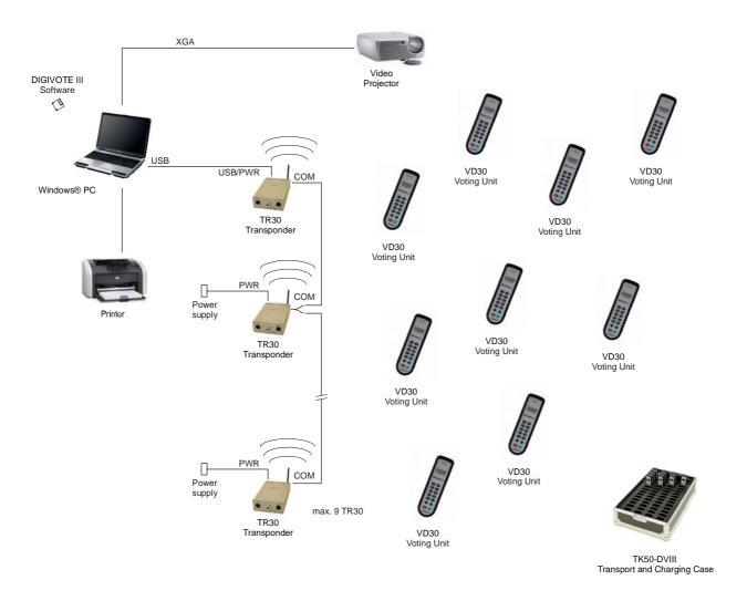
This configuration allows a total distance about 1000 meters. The "inner" transponders are connected by means of special adapters. If required our planning department will assist you.
