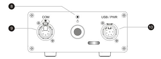
On/Off key - The switch-key is attainable only with a pointed article, so that the switch-key cannot be used by mistake.
