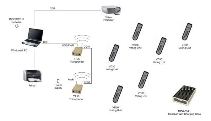
The distance between two transponders may be up to 1000 meters. The transponders are attached via a special cable to the COM interface.
