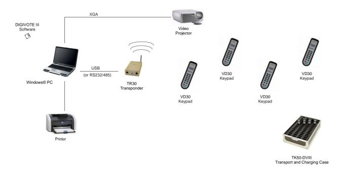
The operating range between the transponder and the voting unit is up to 50m (radius), depending upon the specific location and the building conditions.
