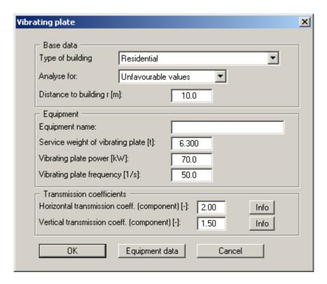
The input corresponds to the input for vibrating pile drivers (see Section 5.2.3.2). However, in addition to power and frequency the service weight of the vibrating plate must be given.
