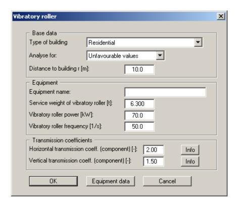
The input corresponds to the input for vibrating pile drivers (see Section 5.2.3.2). However, in addition to power and frequency the service weight of the vibratory roller must be given.
