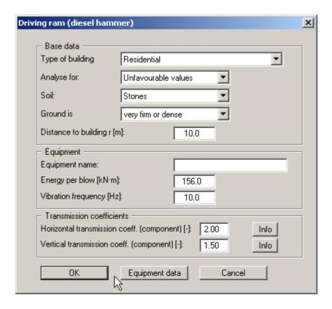
The input corresponds to the input for vibrating pile drivers (see Section 5.2.3.2).
