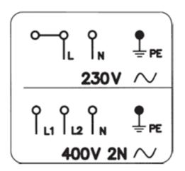
• The cable connections must be in accordance with the diagram located on the bottom of the hob.
