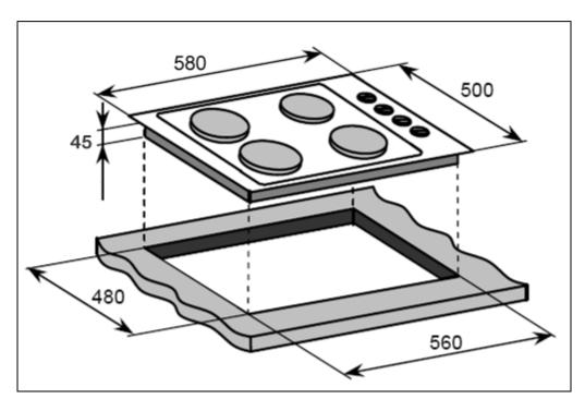
Cut a hole in the worktop that corresponds with the drawing shown above.
