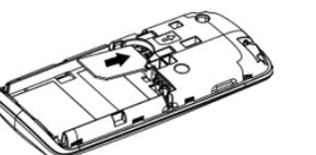
**Installing the Battery**
