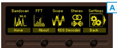
Connect the device to a local network or to the Internet by the applied LAN cable. Through the Front panel navigational menu pressing the "OK" button you will enable you to enter the device main menu (A).
