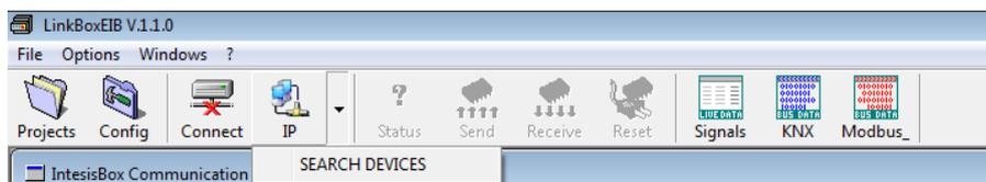
**Figure 6.2** Search IntesisBox when connected to the Ethernet
