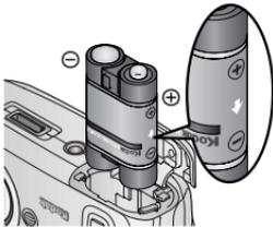
Insert the Kodak EasyShare Ni-MH rechargeable battery pack (included with the Kodak EasyShare camera dock or printer dock) as shown.
