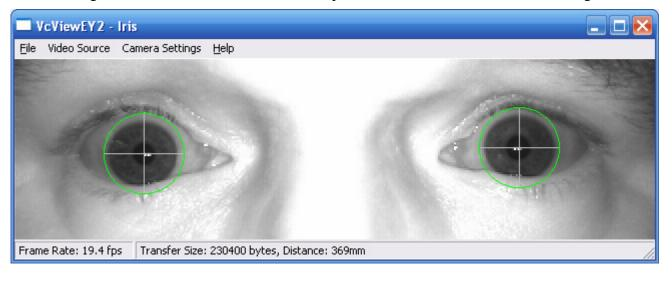
The VcViewEY2 comes with default setting which will allow the device to auto acquire dual iris images when the distance is correct (approx 15 inches from the face), and the iris position and quality is assessed as acceptable. The VistaEY2 device incorporate proprietary Iris Pupil Finding ("IPF"), technology to locate the eyes within the preview stream to allow for the auto acquisition feature.
