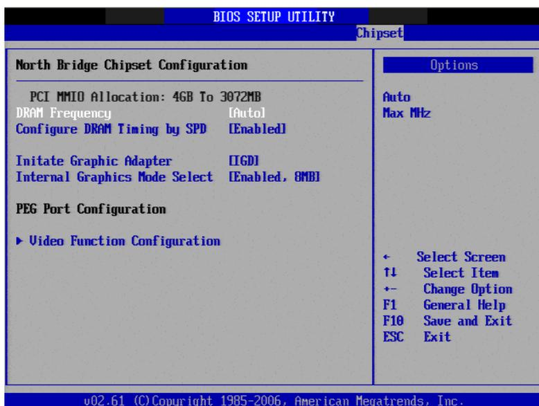
Figure 3.24 North Bridge Configuration
