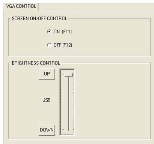
When the application is executed, it will display two blocks of VGA control functions. The application can turn on or turn off the screen shot freely, and it also can tune the brightness of the panels if your platform is being supported. You can test the functionalities of VGA control as follows:
