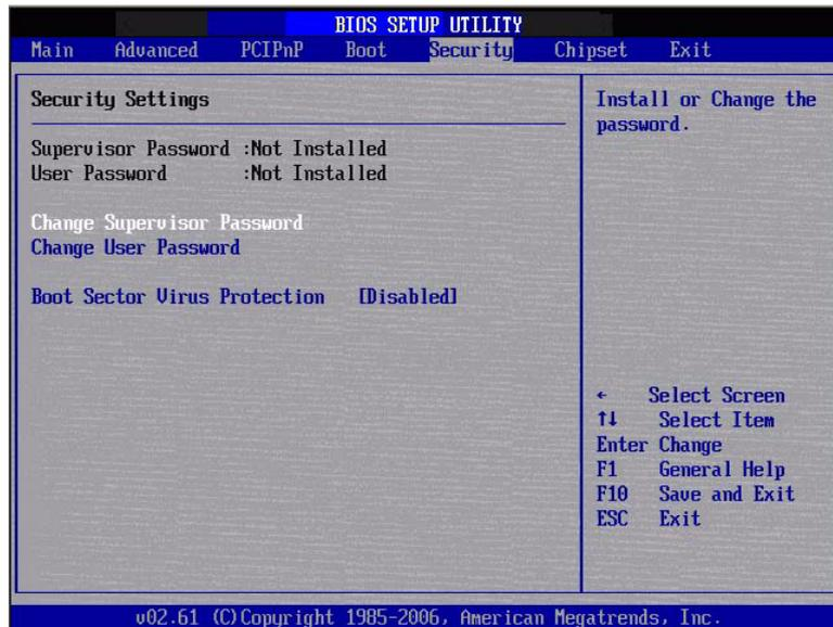
**Figure 3.22 Password Configuration**
