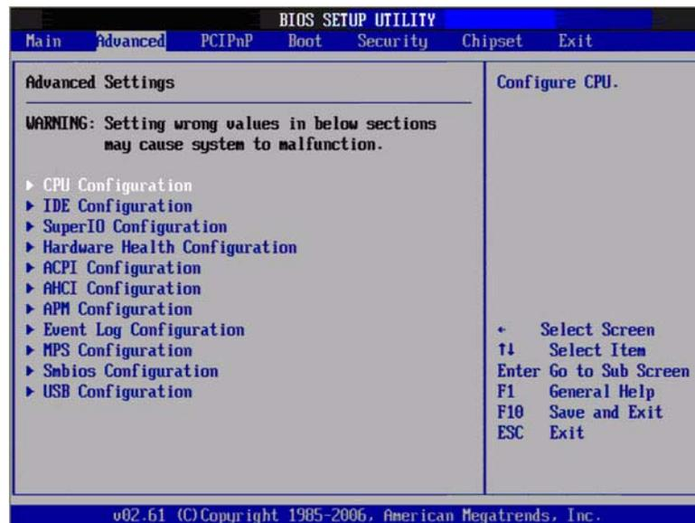
Figure 3.3 Advanced BIOS features setup screen
