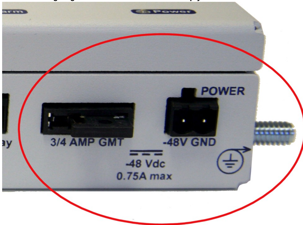
ECU LAN GMT fuse slot, power connection, and grounding lug
