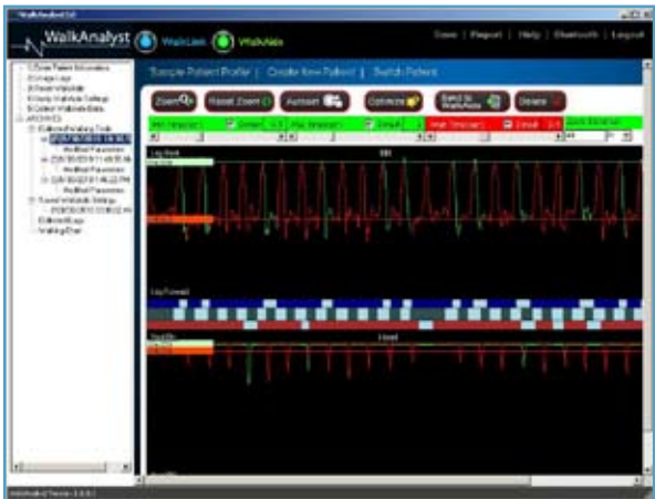
Figure 71: The On Threshold is set too high, creating missed stims
