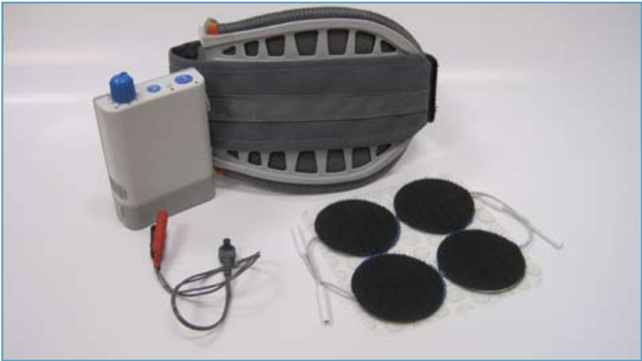
Figure 1: The WalkAide is a functional electrical stimulator designed for people with foot drop
