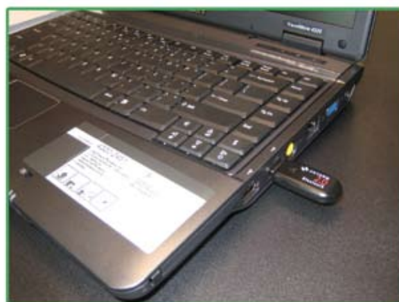
Figure 20: Bluetooth Adapter Hardware Installed
