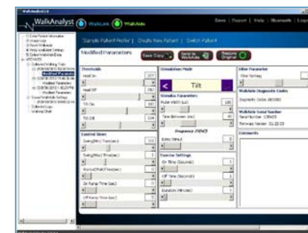
Figure 76: On and Off Thresholds for the Heel and the Tilt Sensors are best adjusted from the date and time stamped graph screens
