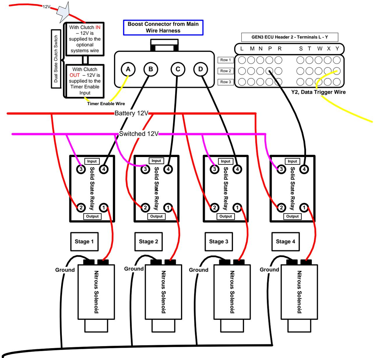
**Solenoid Wiring using the GEN3 Spark Control & Digi-set Nitrous Control**
