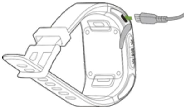
Use only the USB power adapter battery and USB cable provided. Any other USB power adapter and USB cable may cause the explosion of the battery or destroy of the device.
