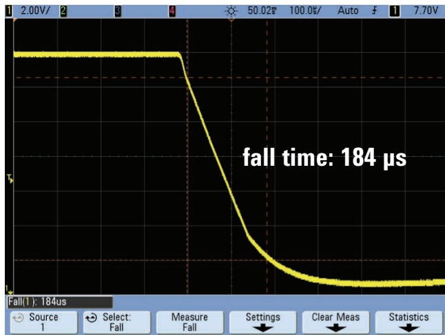
Figure 5. Interrupt pulse fall time measurement of < 200 us
