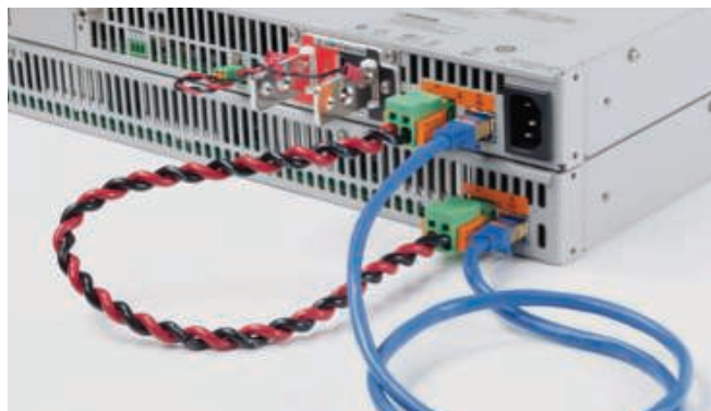
Figure 7. N7909A power dissipater unit rear connections to a 1 kW APS power supply
