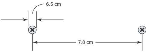
**STEP 2:** Hang the NPort Express on the two screws using the apertures on the ears, and then slide the unit downwards.
