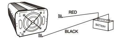
Warning: Only connect to the ac Terminal Block when the inverter is turned off and disconnected from the dc power source.
