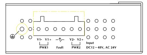
This IVS-2120 provides dual power source for redundancy. The IVS-2120's built-in bridge rectifier output varies in accordance so that the polarity can be ignored. Just pay attention to its power range only.
