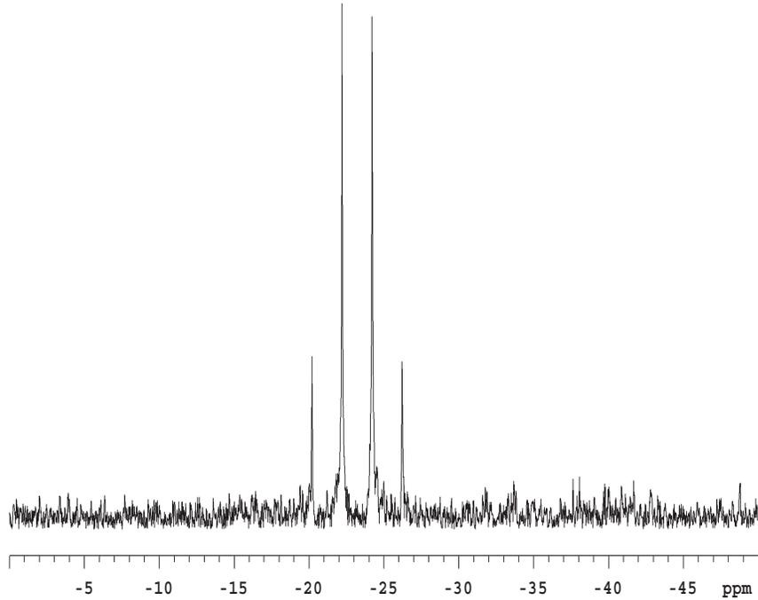
**Figure 21.** Proton Coupled  $^{13}\text{C}$  Spectrum of  $^{13}\text{C}$ -Methyl Iodide
