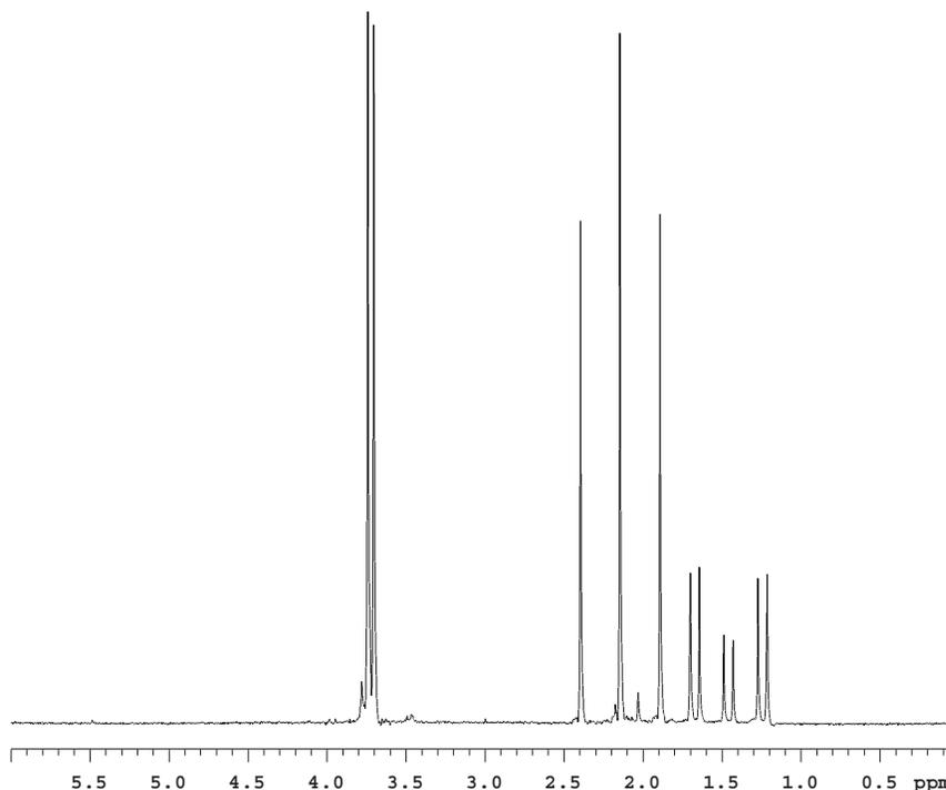
**Figure 16.**  $^1\text{H}$  Spectrum of  $^{13}\text{C}$ -Methyl Iodide
