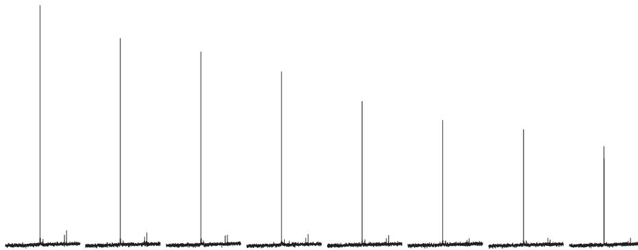
**Figure 24.** Calibration of the Decoupler 90° Pulse Width, pp
