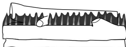
**Figure 26 - Correct Front Burner Flame Pattern**
