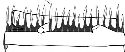
**Figure 27 - Incorrect Front Burner Flame Pattern**
