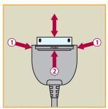
When installing the latching connector support both sides of the connector with your thumb and forefinger (1).
