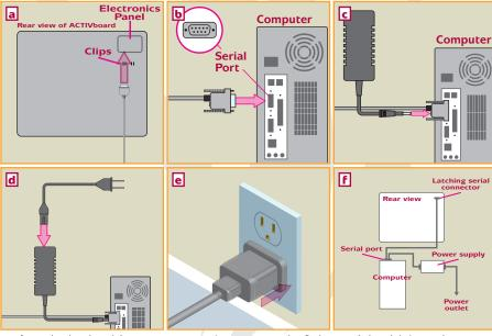
a: Attach the latching connector (on one end of the serial cable) to the larger of the two sockets on the electronics panel (rear top right of the ACTIVboard) and secure the cable to the board with the clip underneath.
