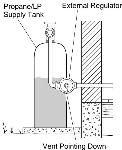
**Figure 13 - External Regulator With Vent Pointing Down**
