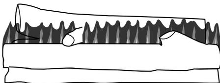
**Figure 27 - Correct Front Burner Flame Pattern**
