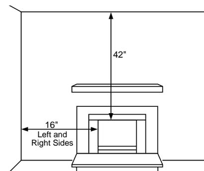
Figure 4 - Minimum Clearance to Wall and Ceiling
