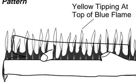
**Figure 28 - Incorrect Front Burner Flame Pattern**
