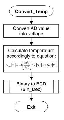
This routine converts value read from AD converter into value in °C units. It is up to user to write code that will handle appropriate accuracy. At the end temperature value is converted into separate digits displayed on LCD. Location: mathpack.inc
