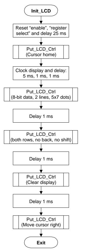
This is a description of how initiation of the display controller is handled. Location: lcd.inc
