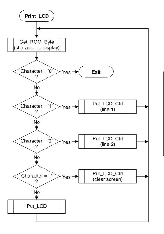
This is the flow for writing a string stored in ROM onto the display. Please not that the string must be null terminated (/0) otherwise the routine won't stop. Note also that digit 1 and 2 is used for determining which line to print on. Location: lcd.inc
