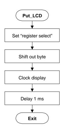
This routine is used for shifting out one byte of display data. Location: lcd.inc
