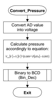
This routine converts value read from AD converter into value in kPa units using appropriate equation. At the end pressure value is converted into separate digits displayed on LCD. Location: mathpack.inc
