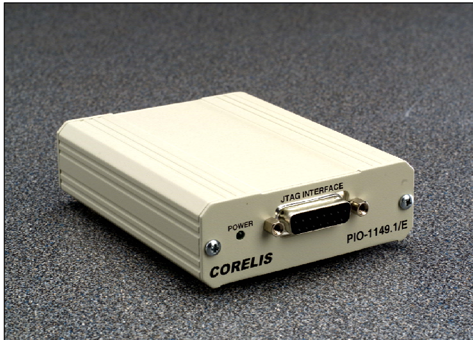
Figure 1-1. The Corelis PIO-1149.1/E Boundary-Scan Controller
