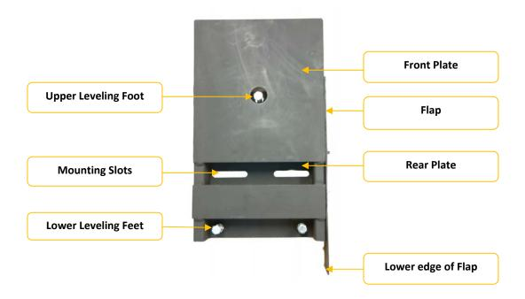
Mounting Slots are used for attaching the Universal Mounting Bracket to the Screed of the paver. ½" bolts, washers, lock washers and nuts are provided to mount the unit.
