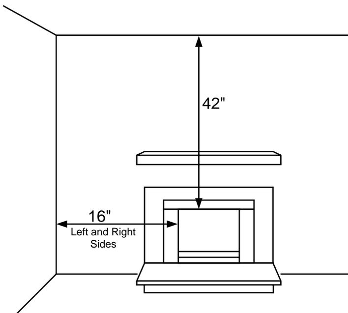
**Figure 4 - Minimum Clearance to Wall and Ceiling**
