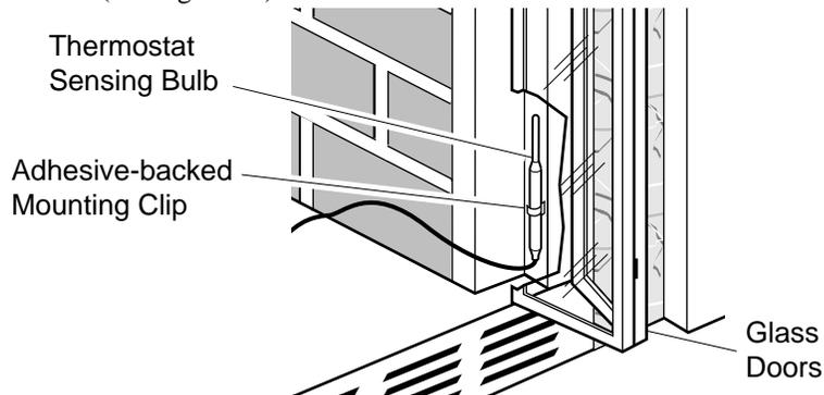
**Figure 31 - Installing Thermostat Sensing Bulb behind Glass Doors**
