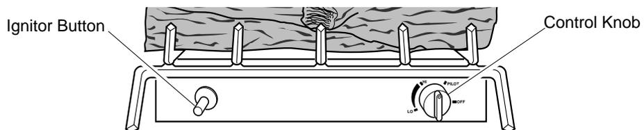
Figure 20 - Control Knob and Ignitor Button Location
