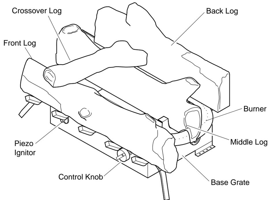
**Figure 1 - Vent-Free Gas Log Heater**
