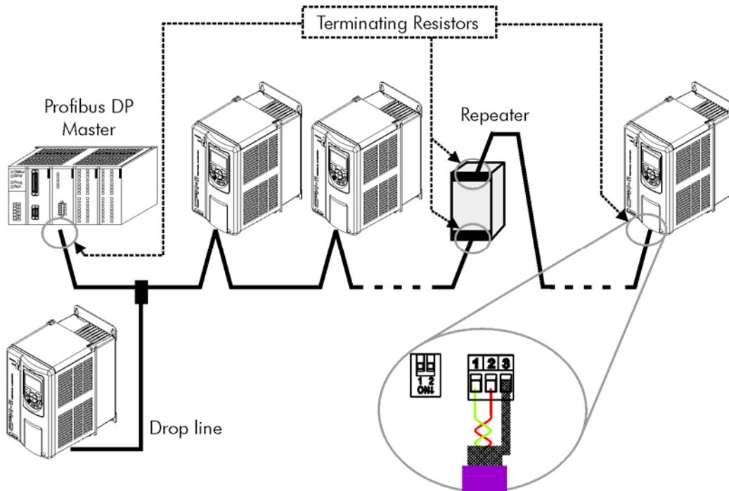
Figure 3.1: Connection example in a Profibus DP network
