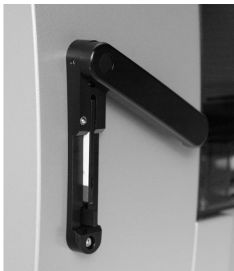
Figure 2. Complete insertion of EZ1 Card. The EZ1 Card must be completely inserted before the EZ1 instrument is switched on.
