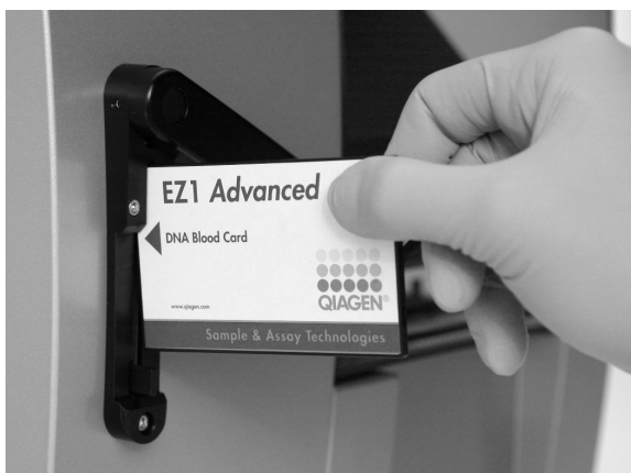
Figure 1. Ease of protocol setup using EZ1 Cards. Inserting an EZ1 Card, containing protocol, into an EZ1 instrument. The instrument should only be switched on after an EZ1 Card is inserted. EZ1 Cards should not be exchanged while the instrument is switched on.
