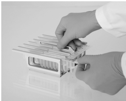
Figure 3. Ease of setup using reagent cartridges. A A sealed, prefilled reagent cartridge. Fill levels vary, depending on the type of reagent cartridge. B Loading reagent cartridges into the cartridge rack. The cartridge rack itself is labeled with an arrow to indicate the direction in which reagent cartridges must be loaded.
