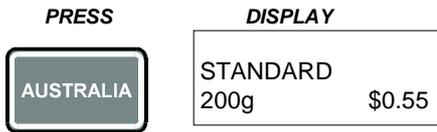
The first line of display confirms the basic service selected and the second line displays the minimum rate of postage for that service.
