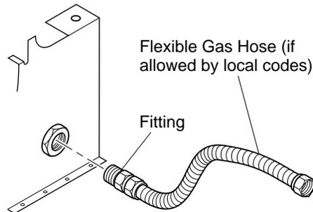
**Figure 10 - Attaching Flexible Gas Hose to Heater**
