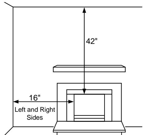
Figure 4 - Minimum Clearance to Wall and Ceiling
