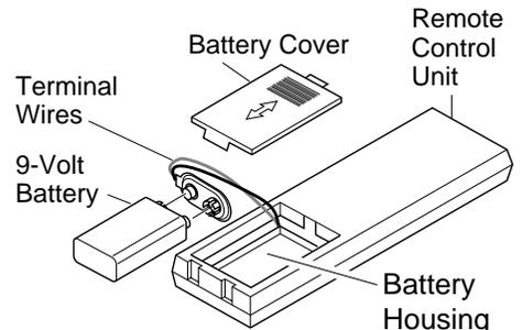
Figure 16 - Installing Battery In Hand-Held Remote Control Unit
