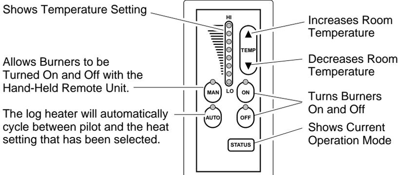
Figure 28 - Thermostat Hand-Held Remote Control Unit Selections
