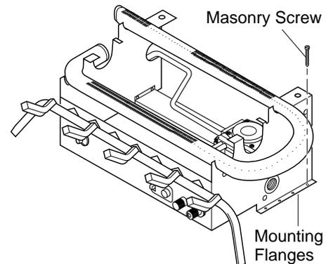
**Figure 11 - Attaching Base Assembly to Fireplace Floor**
