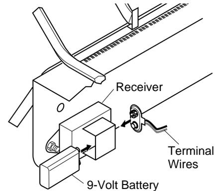
Figure 15 - Installing 9-Volt Battery In Receiver
