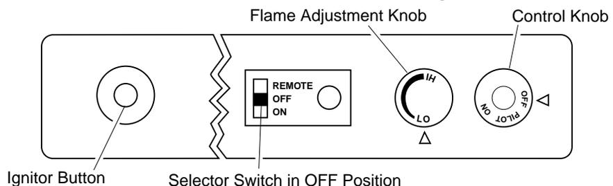
Figure 26 - Control Knob and Ignitor Button Location
