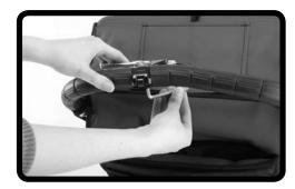
2 To rotate the hand brake's position on the handle bar, loosen the bolt using the supplied Allen wrench. Rotate the hand brake assembly on the handlebar until it is in a comfortable position. Tighten the bolt to secure hand brake.
