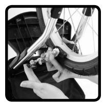
Squeeze the two brake calipers together against the metal rim of the front wheel and flip the black lever forwards to close brake pads.
