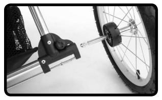
**1** To install, slide the axle peg of the rear wheel into the axle until you hear it click into place. Complete on both sides.
