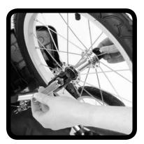
Tighten by turning the wheel lever clockwise while holding the opposite side.
