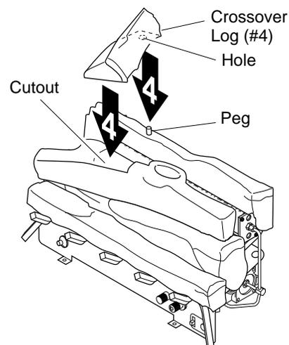
**Figure 20 - Installing Crossover Log (#4)**
