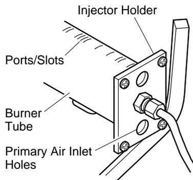
**Figure 29 - Injector Holder On Outlet Burner Tube**
