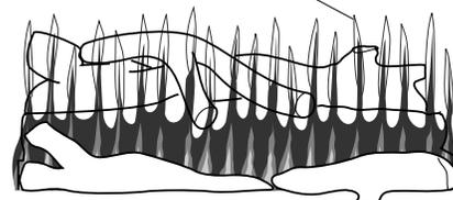
Figure 28 - Incorrect Front Burner Flame Pattern
