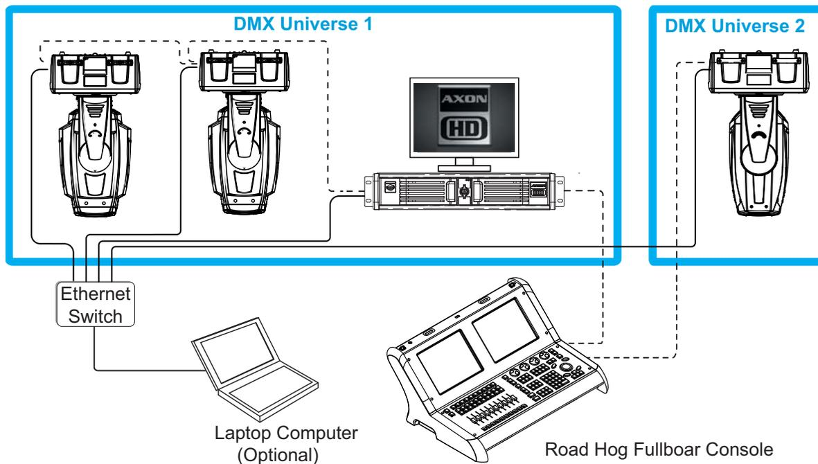
**NOTE:** *If you are using a DMX console and other automated lighting products compatible with Art-Net, this network can also serve as the link for DMX control.*
