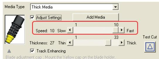
Selecting "Fast" increases the cutting speed, and selecting "Slow" reduces the speed. The slower the cutting speed, the higher the cutting quality. The speed can be adjusted in 10 steps.
