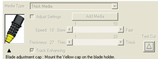
Only the tip of the blade protrudes from the blade holder. The blade adjustment cap color controls the blade length (the protruding length varies according to the color of the cap). The color selection is mostly determined by the thickness of the media to be cut.
