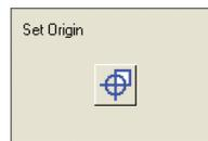
After moving the blade or pen (ballpoint pen) to the desired origin point using the [Blade Position] buttons, click the [Set Origin] button to specify the current position as the origin. This function cannot be used (is not required) when registration marks are used for positioning.
