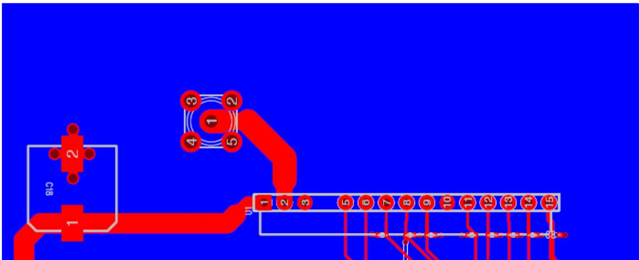
**Picture 7:** Example of lay-out, the connection tracks on PCB on the top side and ground plane in the bottom side.
