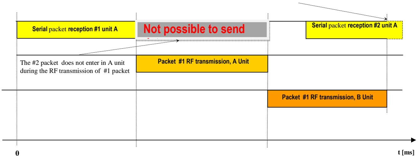
**Picture. 4:** Two data packets transmission
