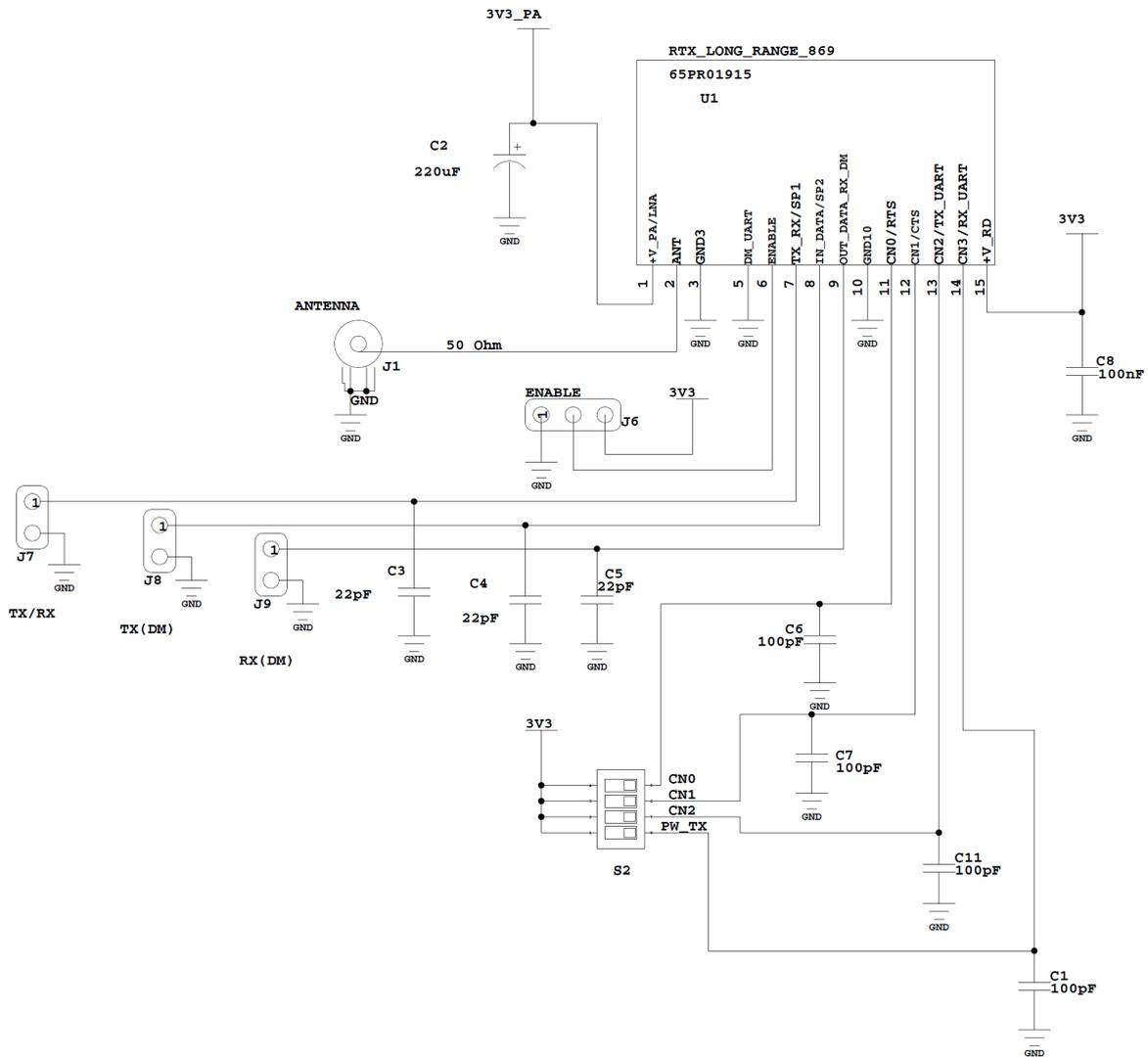
**Picture 4:** Direct-Mode electrical schematic
