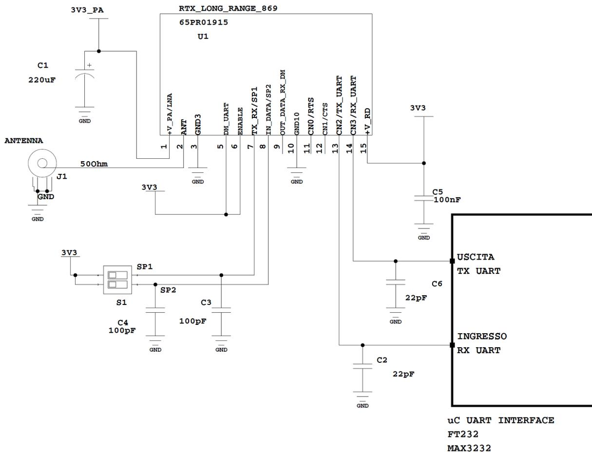
**Picture 5:** Packet-Mode Electrical diagram
