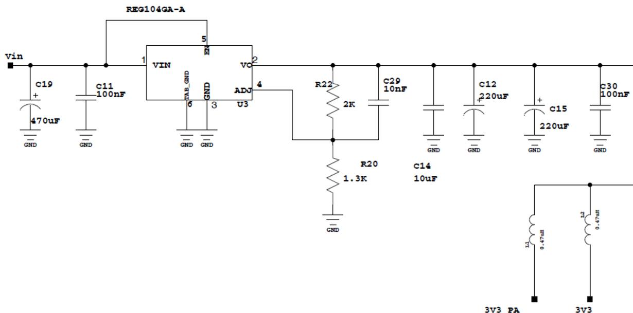
**Picture 6:** Fixed power supply 3V-1A DC-DC
