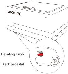
B. Spin the red gear of the Elevating Knob clockwise. You will see that a black pedestal below the Elevating Knob moves down gradually. Continue to spin the red gear until the black pedetal is stabilized on the ground.
