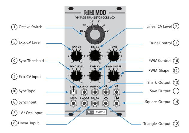
1 Octave Switch: Use the Octave switch to quickly select preset octaves, the Lo setting reduces the oscillator frequency into the Low Frequency Oscillator range so that it can be used as a modulation source.
