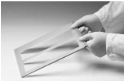
Fig 28. Snapping the cassette.
