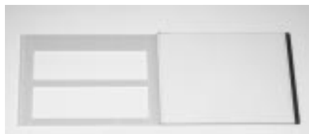
Fig 22. Pre-cast gel cassette open.
