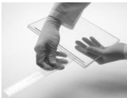
Fig 15b. IPG strip being seated against slab gel.
