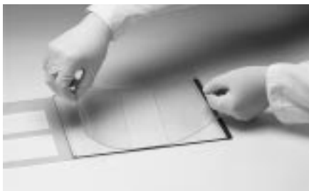
Fig 24. Initial placement of the gel.
