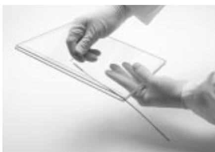
Fig 15a. IPG strip being positioned on cassette.
