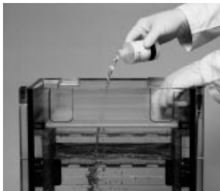
Fig 21. Addition of 100× anode to the separation unit solution.
