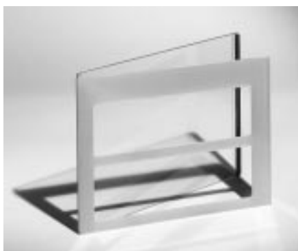
Fig 20. Pre-cast gel cassette.
