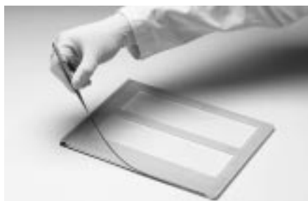
Fig 29. Placing of the IPG strip.
