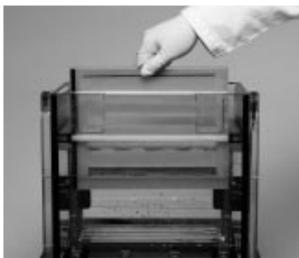
Fig 32. Loading gels into the separation unit.
