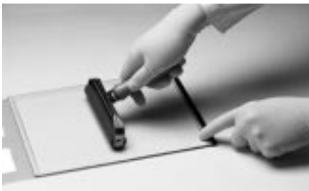
Fig 26. Removing air bubbles.
