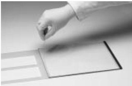
Fig 25. Final placement of the gel.
