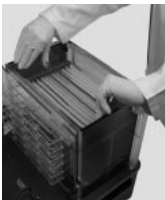
Fig 18. Removing cassettes by hand.
