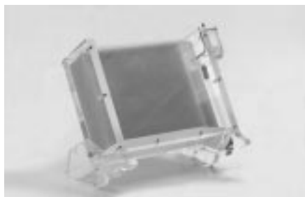
Fig 6a. Gel caster with gel cassettes, tipped back.
