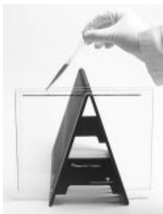
Fig 16. Adding agarose sealing solution.
