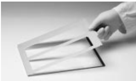
Fig 27. Closing the cassette.
