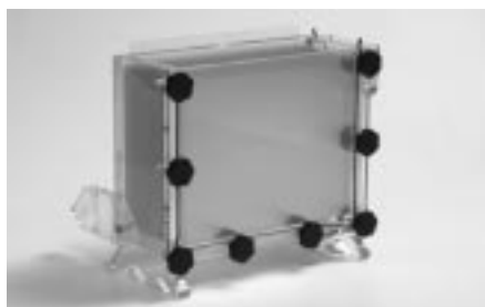
Fig 6b. Gel caster filled and level.
