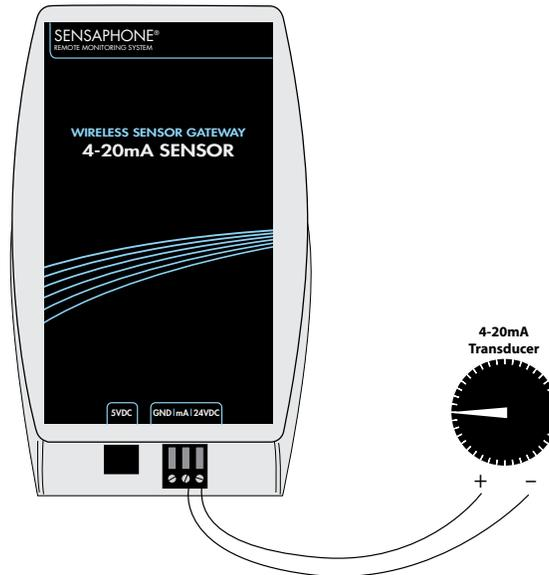
4-20mA Transducer using 24VDC power supply
