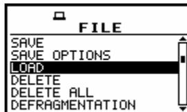
**FILE** list with the **LOAD** text highlighted (displayed inversely)
