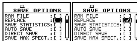
**SAVE OPTIONS** sub-list; the selection of the **REPLACE** in **LEVEL METER** and **1/1 OCTAVE** analyser
