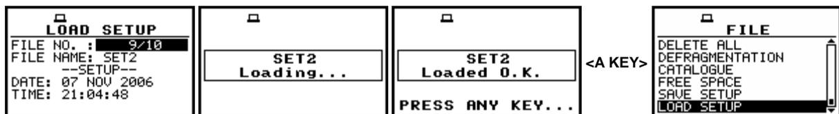
Displays after the execution of the **LOAD SETUP** operation
