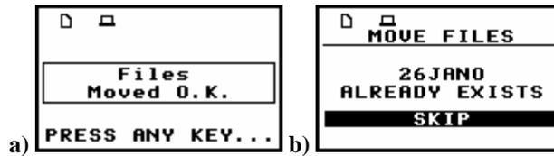
**Display after the execution of MOVE FILES TO USB operation (a) and when the file already exists in the USB memory (b)**
