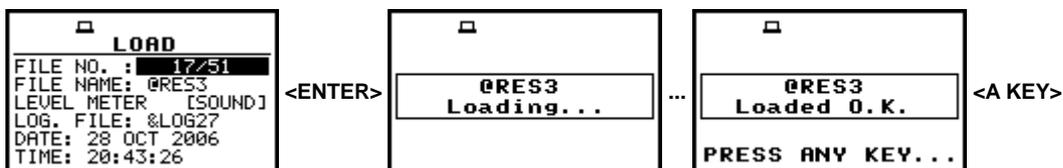
Exemplary displays during a LEVEL METER file loading
