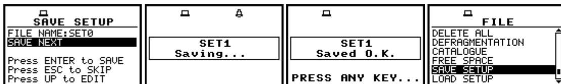
Displays during and after the execution of the **SAVE** operation
