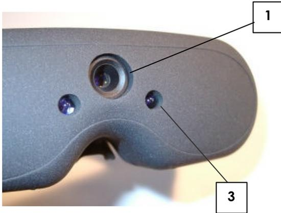
**Two infrared LED's** (3) beside the camera can also be switched on if the light is poor. This additional lighting is virtually unnoticeable to the eye and is not damaging.
