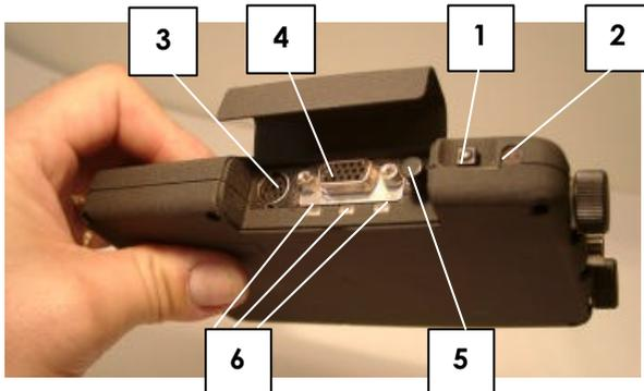
The **push button** (1) for switching on the additional **infrared lighting** and its **control lamp** (2) is situated on the right side of the device.
