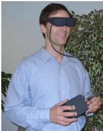
MULTI-VISION consists of the **goggles** and a **power unit with power supply**; a cable connects both parts. The set also includes a main adapter with charger.
