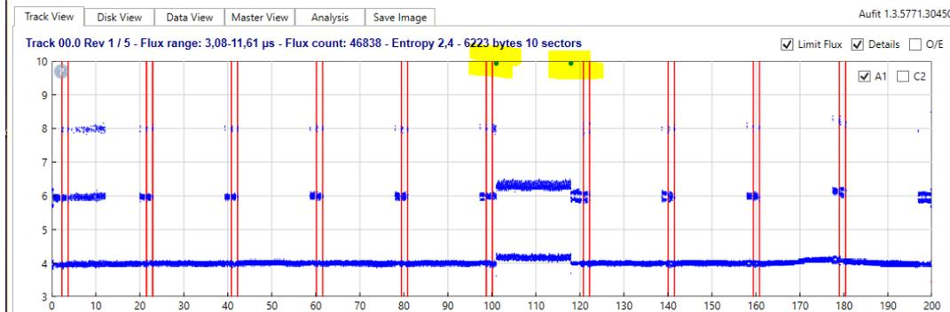
The unprocessed flux transitions (i.e. flux directly read from the file) are displayed as a **scattered chart**. Information about the currently displayed track is displayed at the top of this graph.
