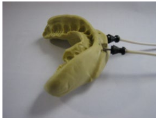
Dental putty probe holder for chronic blood flow measures.
