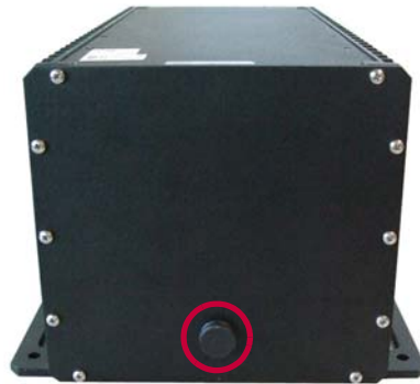
Figure 8. Protective vent on the front plate of the CCA rack
