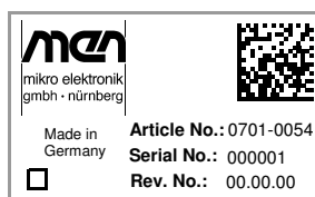
Figure 9. Label giving the board's article number, revision and serial number
