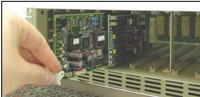
Figure 2-5. 2RU Installation of a Module
