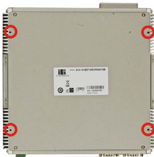
Figure 4-15: Mounting Bracket Retention Screw Holes
