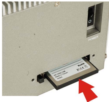
Figure 4-2: CF Card Installation
