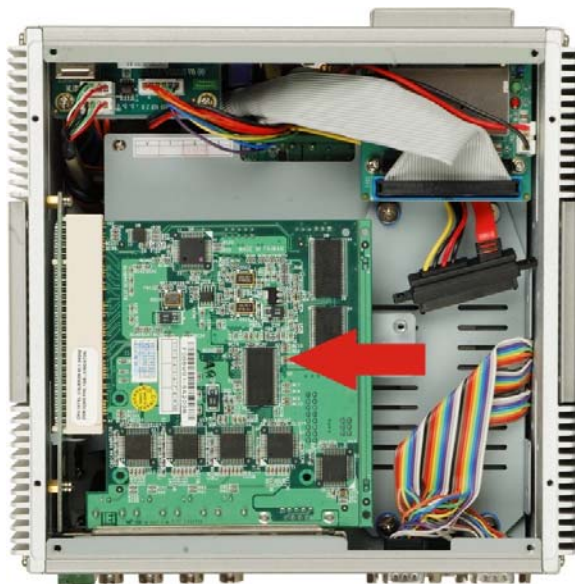
Figure 4-13: PCI Card Installation
