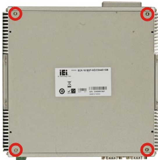
Figure 4-3: Bottom Panel Retention Screws (Bottom)
