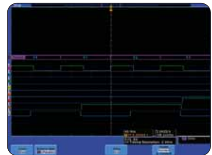
► Clocked parallel bus display, decoding a 7 bit counter.
