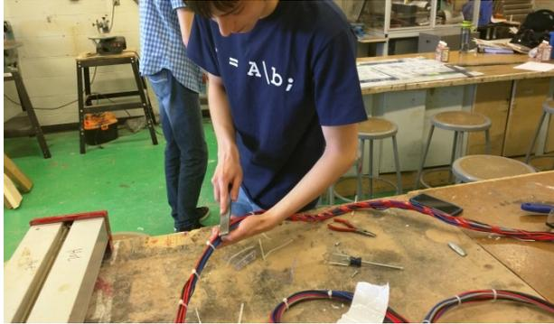
Figure 12 A picture of an employee filing the sharp edges off the tether
