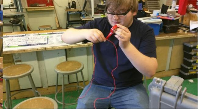
Figure 13 A picture of an employee taping over a soldered wire
