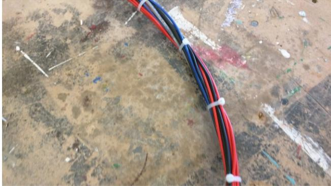
*Figure 11 A picture of the tether connected to the ROV*
